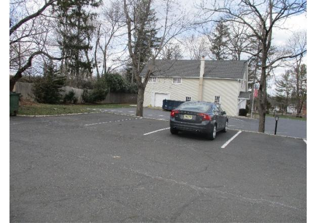
Parking spaces in the parking lot to the west of the building can be converted to porous pavement to capture and infiltrate stormwater runoff from the parking lot. Two rain gardens can be installed in the turfgrass area near the entrance of the building and a third in the rear of the building to capture more runoff from the parking lot. A preliminary soil assessment suggests that more soil testing would be required before determining the soil's suitability for green infrastructure.
