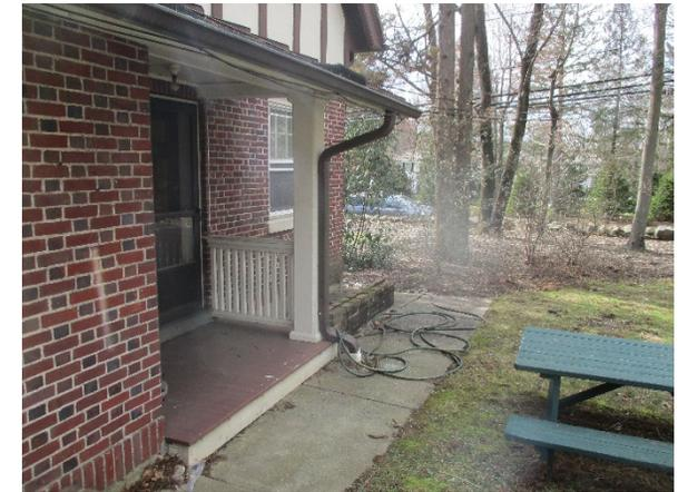
Rain gardens can be installed in the turfgrass area near the entrance of the building and in the rear to capture, treat, and infiltrate stormwater runoff from the parking lot. Downspout planter boxes can be installed to capture and treat stormwater runoff from the rooftop. A preliminary soil assessment suggests that more soil testing would be required before determining the soil's suitability for green infrastructure.
