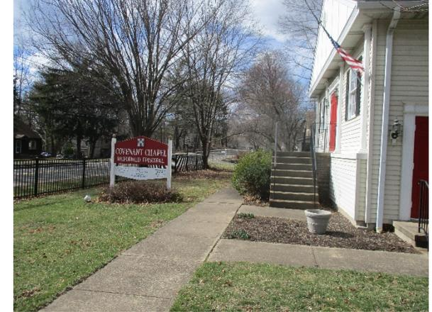
A rain garden can be installed in the turfgrass area near the entrance of the building to capture, treat, and infiltrate stormwater runoff from the roof. This addition could keep rooftop runoff from the storm drain while also enhancing the environment using different colored native flowering plants. A preliminary soil assessment suggests that more soil testing would be required before determining the soil's suitability for green infrastructure.
